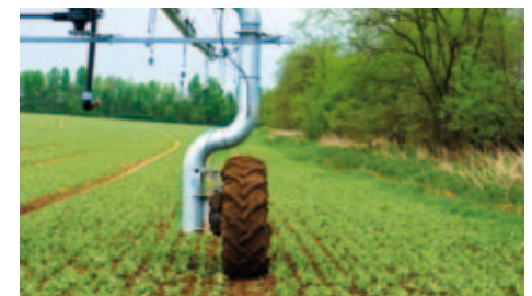
Precise control via guideline as part of underground control system. Drive wheels are rotatable.
