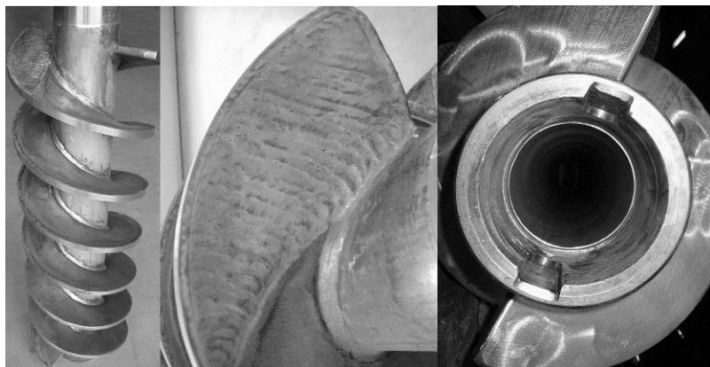
Fig. 13-11 Screw plated with special material and hub mount, new condition
