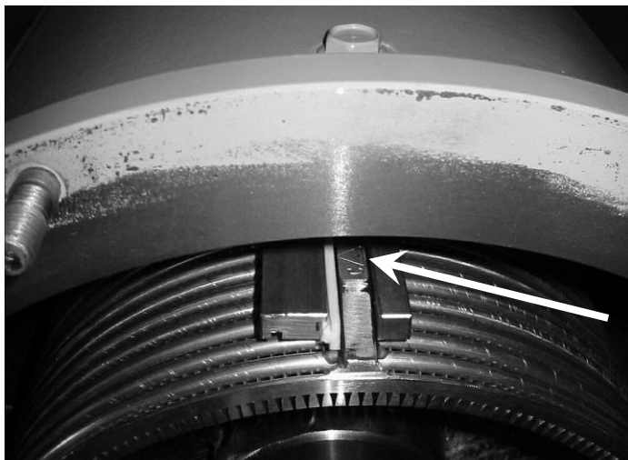
Fig.13-9 Sieve installation position, stamped triangle at top and toward the front of the separator
