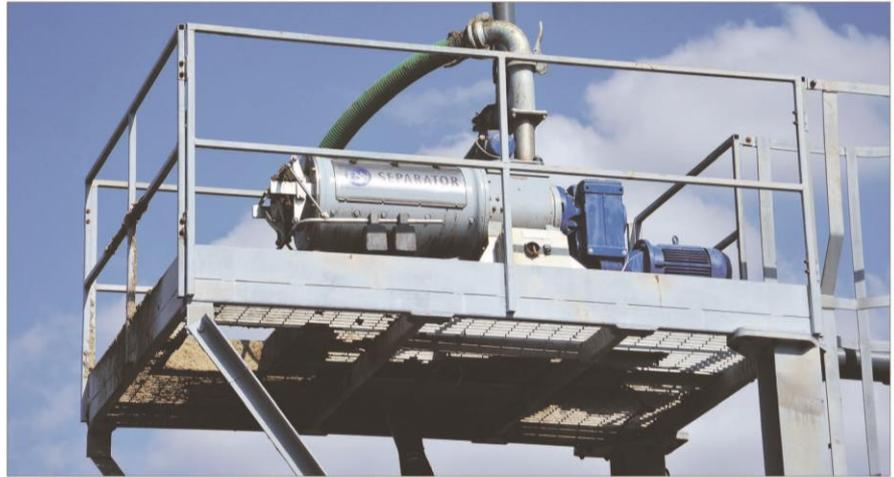
The separator is made by Fan, which is part of the Bauer group, and is powered by a three-phase electrical power supply.
