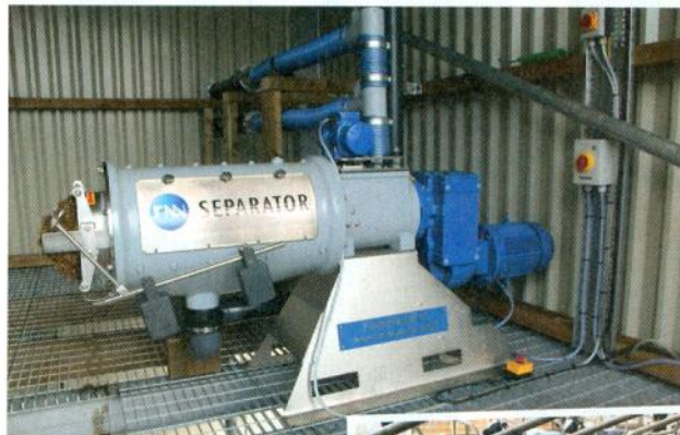
Above: Fibrous material separated from slurry using the FAN Green Bedding machine is used daily as a cost-saving alternative to sawdust, sand and other types of bedding.
