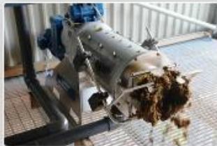
Fibrous Material Separated From Slurry Using The FAN Green Bedding Machine Is Used Daily As A Cost-saving Alternative To Sawdust, Sand And The Like.
