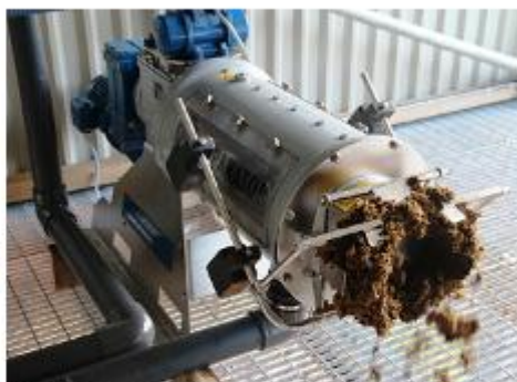
Fibrous material separated from slurry using the FAN Green Bedding machine is used daily as a cost-saving alternative to sawdust, sand and the like.
