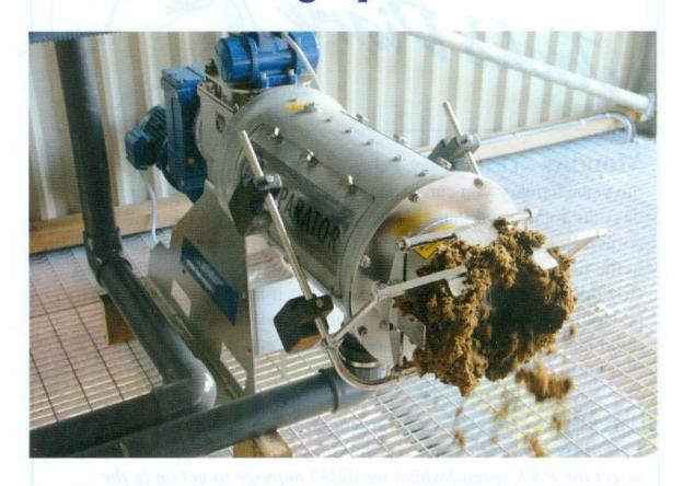
The correct price for the Bauer Green Bedding system pictured here is £40,000 not £200,000 as reported in the January issue of Farm Contractor. Viable for smaller dairy units, the high pressure screw FAN separator produces high dry matter levels in fibrous material separated from slurry. The material produced is ideal for bedding cubicles and the company says, offers a considerable saving over traditional methods and also reduces the amount of slurry.
