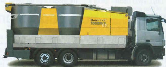
Large 12 t mixes can be produced with the Tourmix Twinpower
