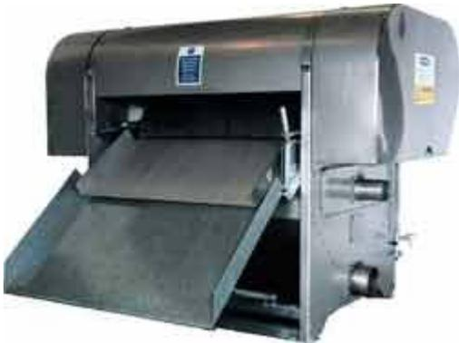
The Carrier Rotoscreen separator from [Linton Solutions](#) also squeezes liquid from solids. But in this case there are two pairs of rollers, one on the inside and one on the outside of a rotating barrel screen.
