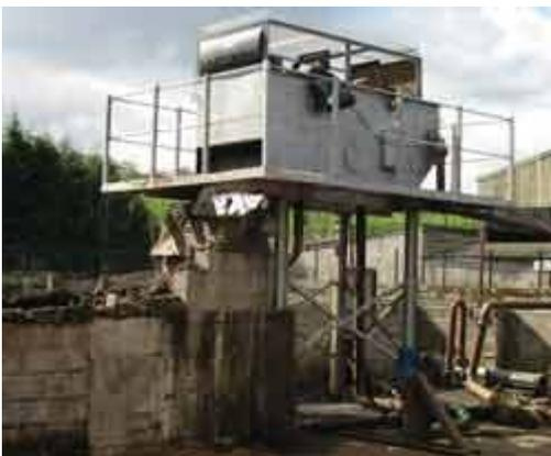
The Groundhog slurry separator from [Pollution Control](#) and the similar unit from [NC Engineering](#) are in the former camp, and have two fixed concave screens with sweeping elements working on the inner surface.
