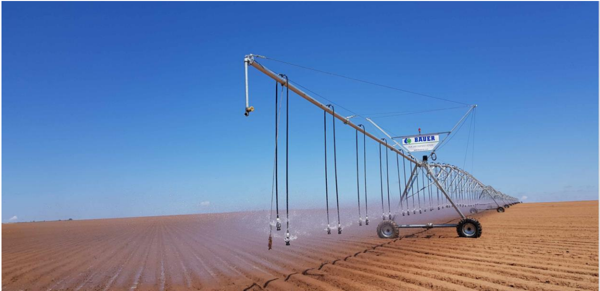
This low-pressure pivot irrigation system irrigates potatoes during the germination phase in Brazil
