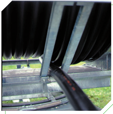
WINDING GEAR The PE pipe is gently layered by a double guided winding mechanism & precisely driven by a helically grooved spindle.
