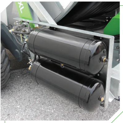
BRAKE (OPTIONAL) For safe road transport, a compressed air brake can also be installed on the Rainstar as an option.
