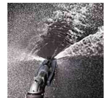
Action of the dynamic jet-breaker
