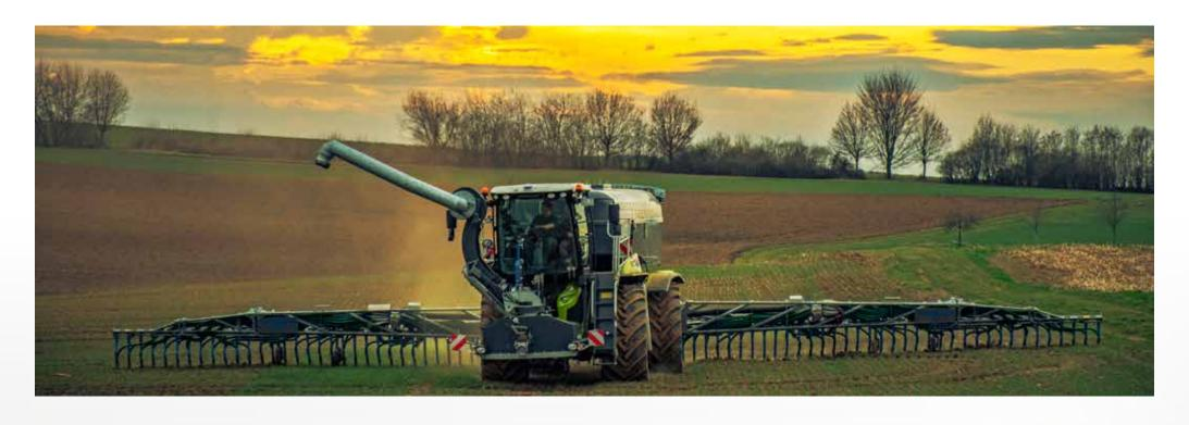
■ Frontunit: 10" pipes, 160° rotation, turbo filler, stone trap box, Vogelsang Rota-Cut RCX-58H with ACC, mounted to front linkage or XERION weight carrier frame, lights, connection tube from frontunit on sideways of cabin, 2x front work lights.
