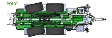
Turning radius 5.7 m smaller (with reference wheel 750/60R30.5)
