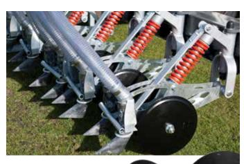
Three-part, ONE-way slit disks enable a precise cutting path and widen the slit for the slurry.
