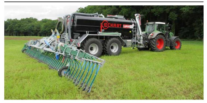
The drag shoe applicator has specially shaped drag shoes that open up the crops and deposit the slurry directly on the ground. The 40 mm wide flow hoses are evenly supplied via one or two Bomech distribution heads and positioned at 25 cm intervals. A slope compensation system optimally adapts the individually spring-loaded drag shoes to the terrain. Undesired dripping is prevented by swinging the flow hoses to an upward position.
