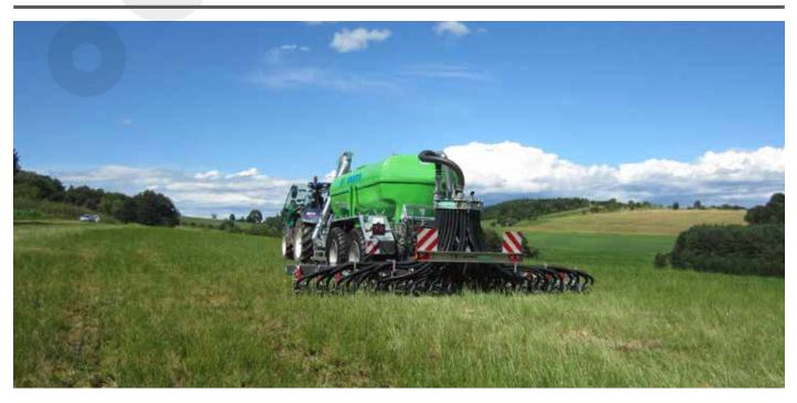
The lightweight disk injector is specially designed for attachment to slurry tankers to keep the empty weight of the slurry tanker as low as possible. The 50 mm wide flow hoses are evenly supplied by a central distribution head and deposit the slurry in slit rows 20 cm apart. The 305 mm, three-part disks open up 2-6 cm slits in the ground and are arranged in disk pairs. Each disk pair is equipped with caster steering and a mechanical drip stop.
