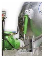
Top trailer fixation (standard fixation)
