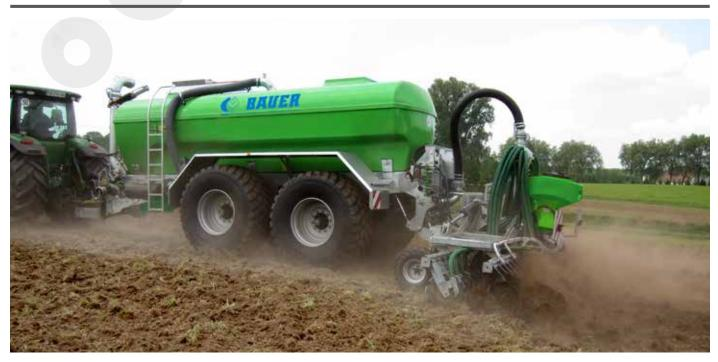
The Cerres S disk harrow works the slurry into the ground in a single step. The two rows of toothed disks introduce the slurry into the ground gently, in a flat profile. Maintenance-free bearings and a disk diameter of 510 mm make the Cerres S an economical machine that was designed specifically for attachment to slurry tankers.
