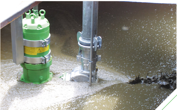
FEEDING OF THE SYSTEM WITH A SPECIAL SUBMERSIBLE MOTOR CHOPPER PUMP
