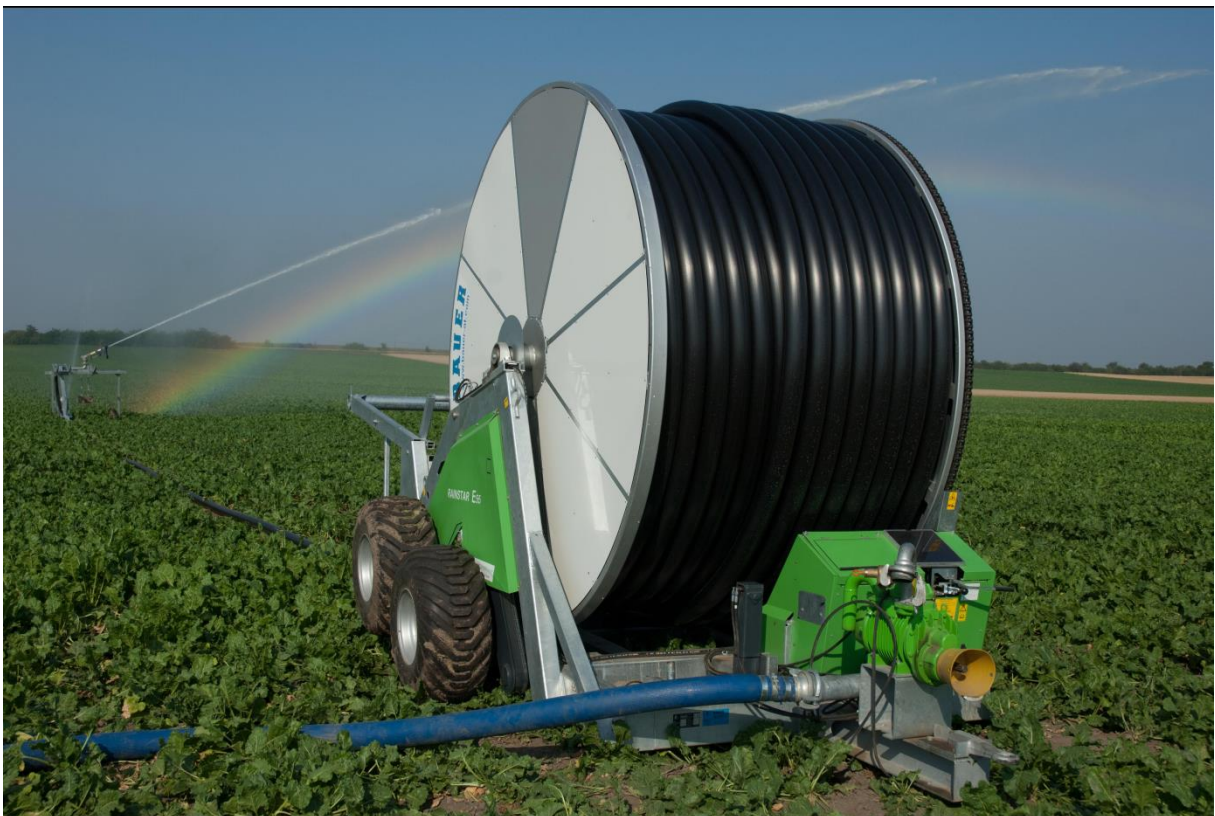
The hose reel irrigator is a classic irrigation machine. This Rainstar E55 is irrigating sugar beets.
